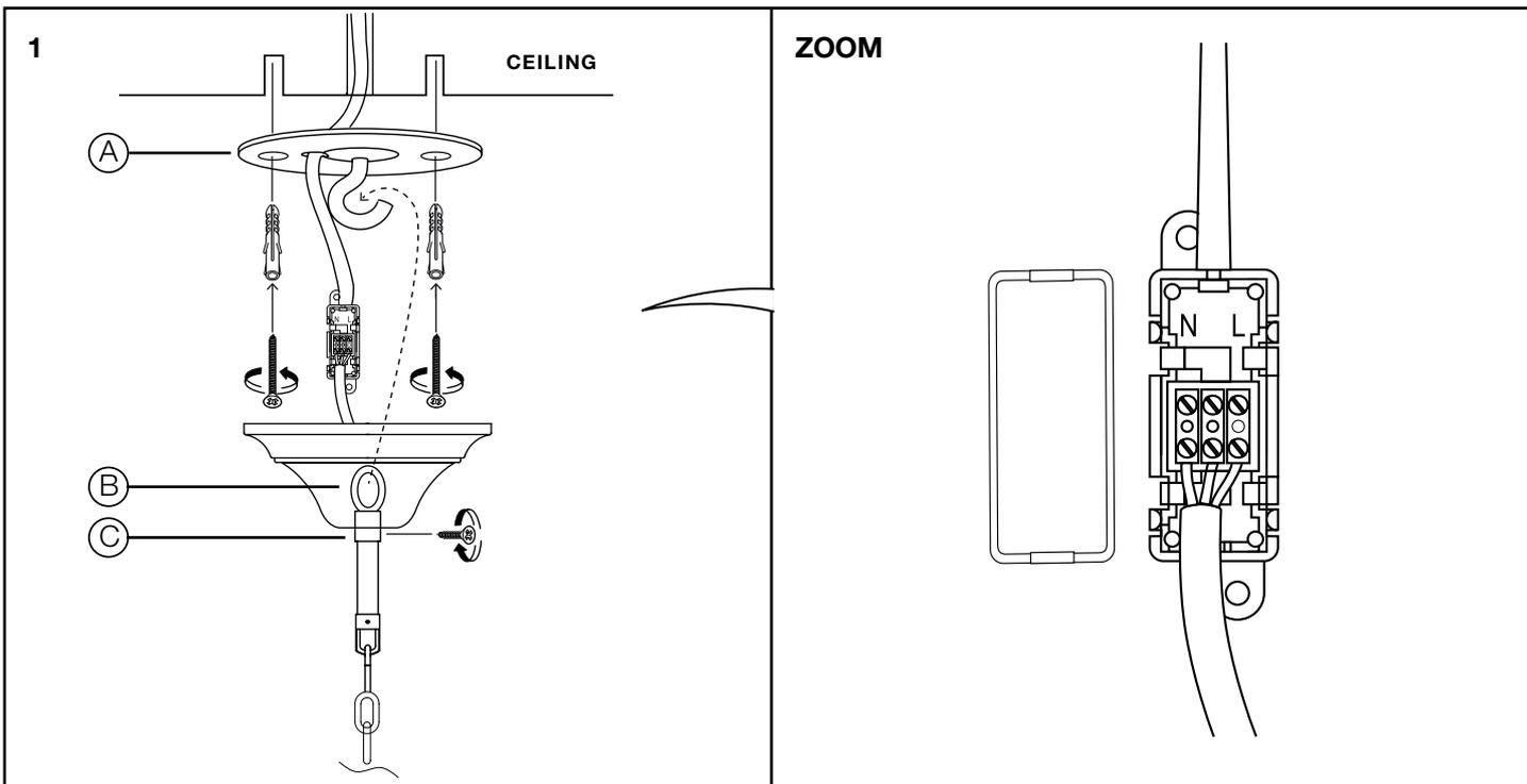
Turn off the electricity supply at the main circuit panel before installing.
